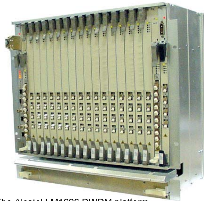
The Alcatel LM1626 DWDM platform
