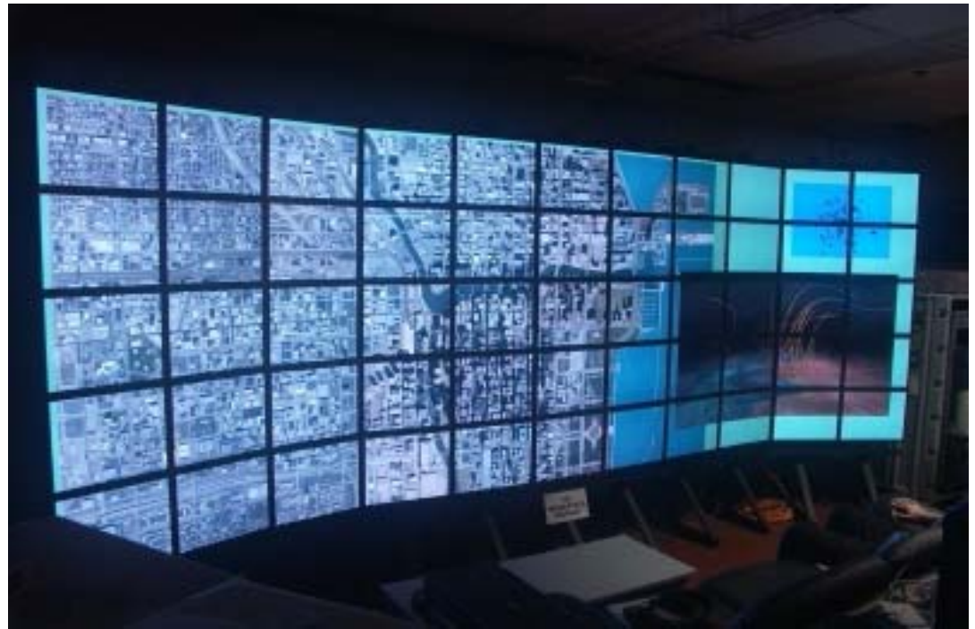
A "LambdaVision" display, using 55 LCDs Resolution: 17.600 x 6.000 pixels
